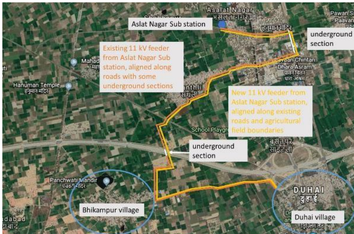
Figure 10: Duhai Feeder Incomer from Aslat Nagar Substation in Ghaziabad Zone, DVVNL
