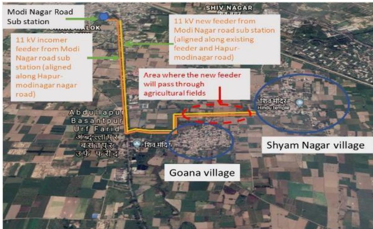
Figure 8: Goana Shyam Nagar Feeder (incomer from 33/11 kV Modinagar Road Substation) in Bulandshahar Zone in DVVNL
